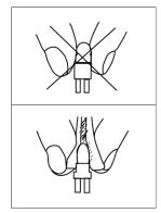
**DISCHARGE LAMP WARNING**: This fixture is fitted with a discharge lamp, which is highly susceptible to damage if improperly handled. Never touch the lamp with your bare hands, as the oil from your hands will shorten lamp life. Also, never move the fixture until the lamps have had ample time to cool. Remember, lamps are not covered under warranty conditions.
