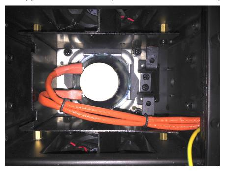
10. Replace the lamp cover back into place by securing (4) screws marked "A", "B", "C", and "D".
