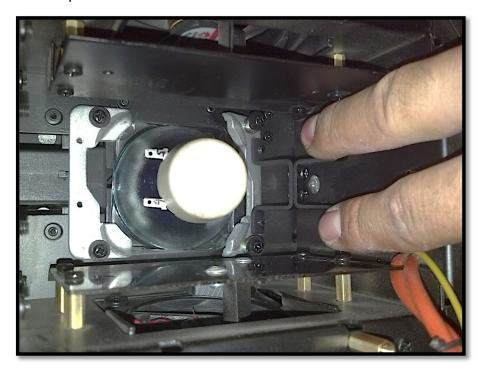
4. While pulling the retention handle with your **RIGHT** hand, use your **LEFT** hand to gently twist the lamp **COUNTERCLOCKWISE** to remove it from under the retention brackets.
