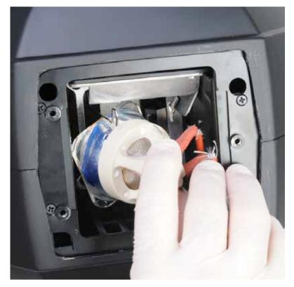
3. Gently remove (2) Wires connected to spade terminals on base of lamp.
