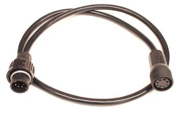
**ELAR Q1 IP EXTENSION CABLE 9.8 ft. (3m) - SKU# 60413990038 (NOT INCLUDED)** IP rated 9.8 ft. (3M) power/data extension cable with 8pin male and 8pin female ends, used to daisy chain up to (10) **ELAR Q1**<sup>™</sup> fixtures.
