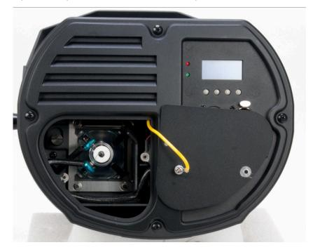
3. Gently remove (2) Black Wires connected to spade terminals on base of lamp.
