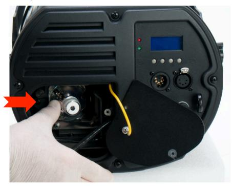
8. Make sure the lamp is properly seated into place just like the old lamp was.
