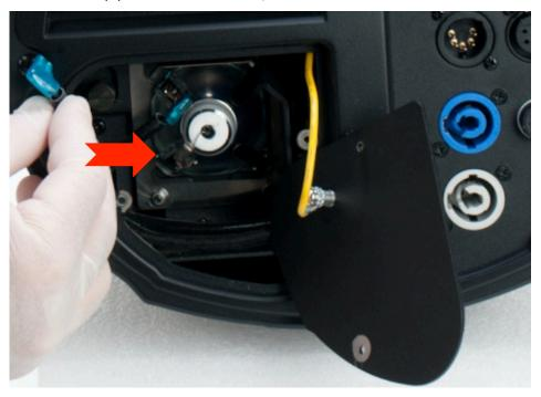
**10.** Make sure each wire is securely attached to the lamp.
