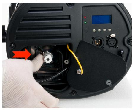
5. Once lamp is released, grab the lamp base with your thumb and index finger and gently pull the lamp **OUT** towards the **LEFT** and **AWAY** from the fixture.
