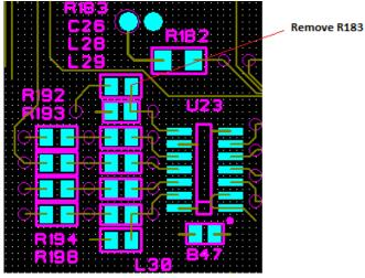
(E) Install one  $330\Omega$  0805 resistor (HES part number 90121040EF) at reference designator R183.
