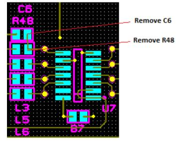
(E) Install one  $330\Omega$  0805 resistor (HES part number 90121040EF) at reference designator R48.
