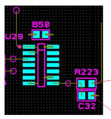
Install 330 ohm 0805 Resistor in R223 20121040EF
