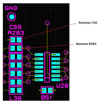
(N) Install one  $330\Omega$  0805 resistor (HES part number 90121040EF) at reference designator R283.
