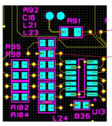
Install 330 Ohm 0805 Resistor in R92 90121040EF
