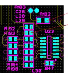
Install 330 ohm 0805 Resistor in R183 90121040EF
