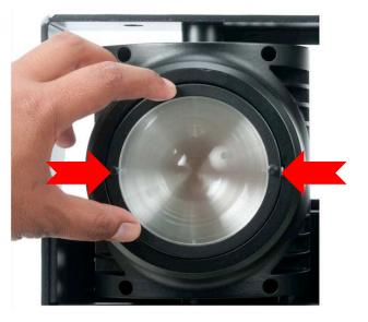
**3.** While applying gentle pressure against the lens, slowly turn the lens counter-clockwise a ¼ turn, until both small black raised plastic tabs are positioned vertical at 12 and 6 o'clock. (See image
