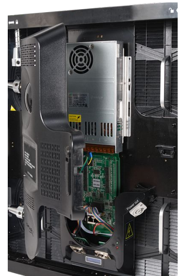
AV6: Power Supply Panel—Opened
