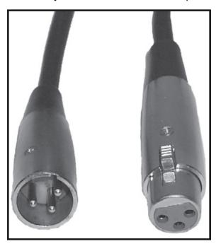
**Notice:** Be sure to follow the diagram below when making your own cables. Do not use the ground lug on the XLR connector. Do not connect the cable's shield conductor to the ground lug or allow the shield conductor to come into contact with the XLR's outer casing. Grounding the shield could cause a short circuit and erratic behavior.
