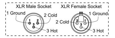
**Special Note: Line Termination.** When longer runs of cable are used, you may need to use a terminator on the last unit to avoid erratic behavior. A terminator is a 110-120 ohm 1/4 watt resistor which is connected between pins 2 and 3 of a male XLR connector (DATA + and DATA -). This unit is inserted in the female XLR connector of the last unit in your daisy chain to terminate the line. Using a cable terminator (ADJ part number Z-DMX/T) will reduce the risk of erratic behavior.
