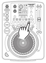
**TRANS/PAN EFFECT:** The Trans effect simulates a real-time mixer transformer effect. When the "Transformer" effect is activated the TRANS LED will flash green, when the "Pan" effect is selected the PAN LED will flash blue. The Pan effect allows you to pan the output from the left channel to the right channel.
