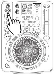
2) Press the IN BUTTON (26). This will set the starting point of the SEAMLESS LOOP. The IN BUTTON (26) LED will flash then glow.
