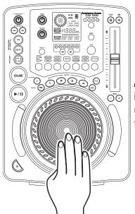
**IN CUE MODE:** While in cue mode and when the touch sensitivity function is active, tapping on the *JOG WHEEL (13)* can be used to start playback. The unit will continue to playback until the *JOG WHEEL (13)* is released. Once the *JOG WHEEL (13)* is released the unit will return to the last cue point.
