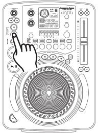
3) Press the OUT BUTTON (24) to set the ending point for your SEAMLESS LOOP (Figure 20). The IN BUTTON (26) and OUT BUTTON (24) LEDs will immediately begin to flash rapidly, indicating the SEAMLESS LOOP mode has been activated.
