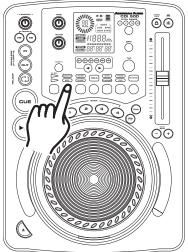
**ACTIVATING TOUCH SENSITIVITY:** Before you can use the *JOG WHEEL* (13) to control the play and cue commands you must first activate the jog wheel touch sensitivity. To activate the touch sensitivity mode, be sure the *FX SELECT LED* (21) is glowing green. Once the *FX SELECT LED* (21) is glowing green, press and hold the *SCRATCH BUTTON* (19) until it begins to flash red repeatedly. This will activate touch sensitivity mode.
