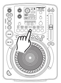
**HOLD BUTTON:** Use the HOLD BUTTON (19) to lock your customized parameters. If the hold button is not activated any changes to your parameters will be momentary. To activate the hold function press the HOLD BUTTON (19) as in figure 50. When the hold function becomes activated, the hold button will begin to glow red.
