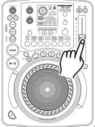
**Using the Pitch Slider (7):** Be sure the pitch function has been activated as described above. To use the *PITCH SLIDER (7)* slide the slider up and down. Down will increase the pitch and up will decrease the pitch.
