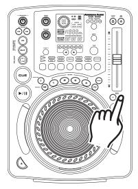
Holding down or tapping on the (-) PITCH BEND BUTTON (11) will provide a slow down in the playback pitch.
