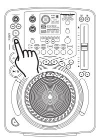
**REPLAY LOOP** - The *RELOOP* (22) function allows you to return to your stored loop at any time. The *IN BUTTON* (26) and *OUT BUTTON* (24) LEDs will indicate a loop is stored in memory, and may be played at any time. To replay the loop, press the *RELOOP BUTTON* (22). The *IN BUTTON* (26) and *OUT BUTTON* (24) LEDs will again begin to flash indicating SEAMLESS LOOP mode has been activated and your stored loop will immediately begin to play.
