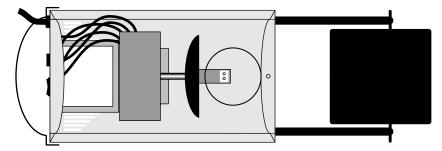
Remove the lamp from the socket and insert a new one as illustrated above.
