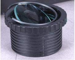
When the lens "pops" out, the picture to the left is what you should see. Remove the lens and retainer ring.
