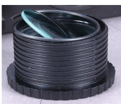
Flip the focus lens barrel over and insert the 52 degree lens. Carefully insert the retainer ring. Please do this very carefully. Make sure retainer ring is in correctly, flesh against the lens. Now you can screw the focus lens back into the H2O LED.
