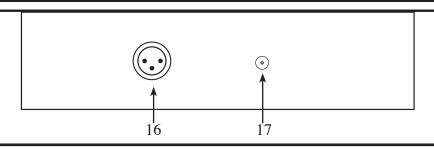
16. DMX OUT - Used to send DMX signal to the compatable LED fixtures.
