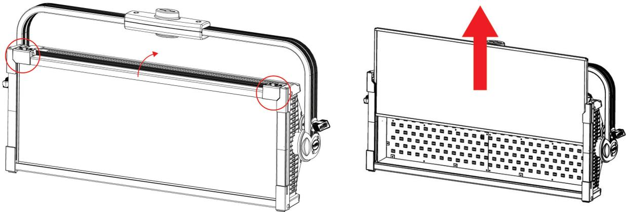
2. Slide the Intensifier Lens into the slot. **Please note that the Intensifier Lens is NOT reversible. The forward-facing side of the Intensifier Lens should have a slight ridge in the lens frame, while the rearward-facing side should have a smooth lens frame.**
