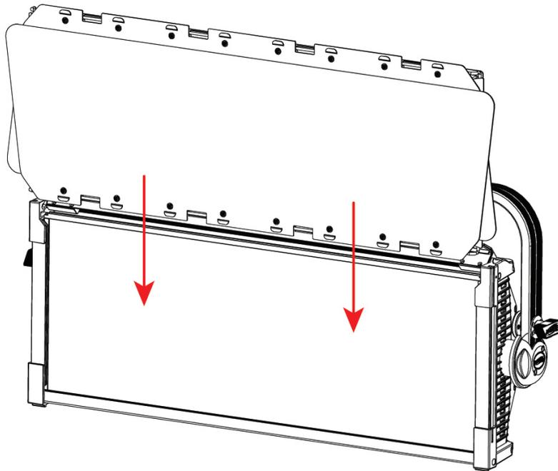
3. With the barndoors locked securely in place, pull on the tabs at the edges of the barndoor flaps to deploy the barndoors. Installation is now complete. **Please note that the barn-door accessory must be installed with its own safety cable! Refer to the diagram in the Fixture Installation section of this manual.**
