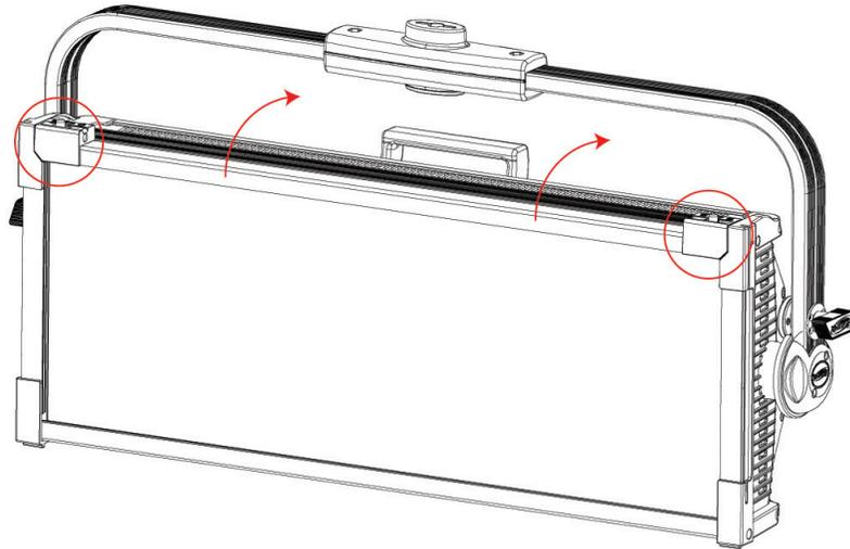
2. Look beneath the frame lock tabs and locate the installation slots on the inner edge of the frame. The slot closest to the front of the device should be vacant. Carefully slide the barndoor into this slot, then flip down the top edge of the frame and lock the frame lock tabs back in place.
