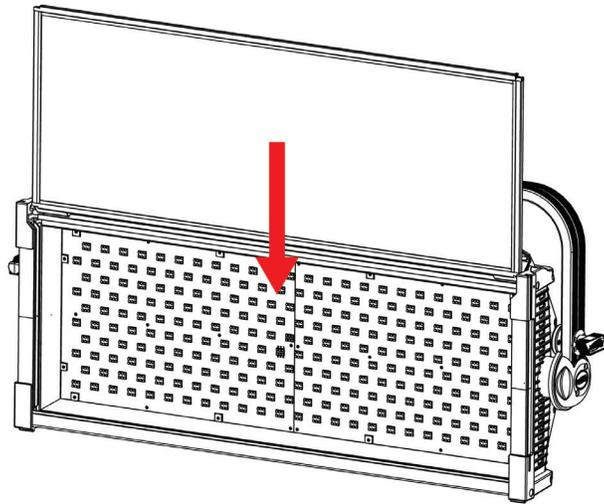
3. Flip the top edge of the fixture frame back down into place, and lock the frame tabs back into place. The installation is now complete.
