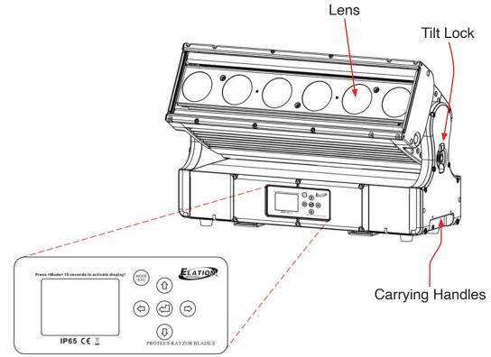
LCD Display & System Menu Controls
