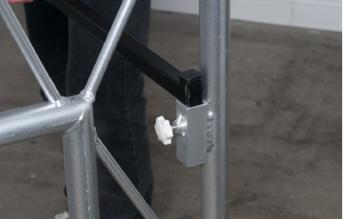
5. Hand tighten the (4) thumb screws located on the support bar slots on both ends of the table.
