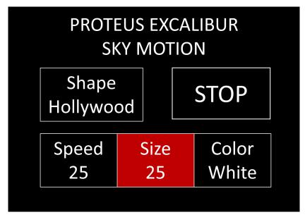
If the screen is locked, hold "MODE" for 10 sec until the countdown is completed. Select one of the available shapes in the top left box. Use the arrow keys to navigate, noting that the current selection is indicated by the red highlighting, then press "ENTER" to select. Use the Up/Down arrows to browse the shapes and preview the results.
