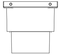
1. Mount and secure the internal multi-use mounting-bracket to the junction-box.
