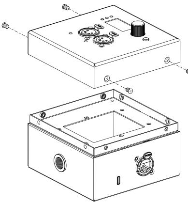
2. Remove the (4x) hex-screws securing the integrated multi-use mounting-bracket to the mounting case. This will be used to mount to the control panel.
