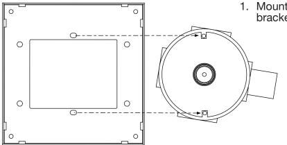
1. Mount and secure the internal multi-use mounting-bracket to the junction-box.
