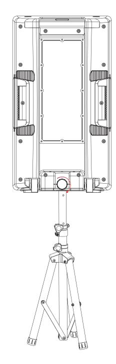
Use the two carry handles mounted located on both sides of the rear panel to carefully lift the speaker and lower it onto a compatible mounting device.
