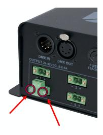
Begin by inserting the male end of the Phoenix connector into the desired signal output port on the driver, making sure that the latch on the Phoenix connector engages with the signal output port. Tighten the two screws located to each side of the wire terminals, as highlighted in the image to the above right.
