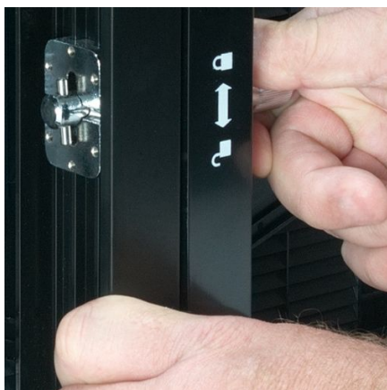
2. Compress spring of panel connector and pass locking-tab through tab-keyed connector socket
