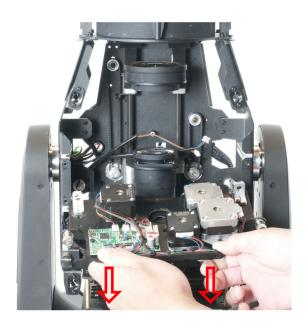
6. Loosen the thumb screws for the gobo wheel module, and carefully slide the gobo wheel module out of its mounting slots. Place the module on a flat, stable surface in a DUST-FREE, INDOOR location.
