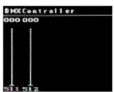
With **Program** selected, use  $\uparrow \downarrow$  to navigate between **Edit**, **Fade**, **Speed**, and **RunSet**. Starting with **Edit**, use  $\longleftrightarrow$  to change **Step##** from 00 to 19, then pressing <Enter>  $\longleftrightarrow$  brings you to the **DMXController** screen for that **Step**. Use  $\longleftrightarrow$  to navigate to the desired channel (001 to 512), then use  $\uparrow \downarrow$  to change the channel value (000 to 255).
