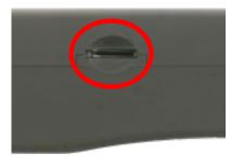
1. With the software update stored on the MICRO SD card, insert the SD card into the slot located at the left side of the C-Loader II.
