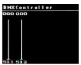
Selecting **DMXOut** brings you to the **DMXController** screen. Use  $\longleftrightarrow$  to navigate to the desired channel (001 to 512), then use  $\circlearrowleft$  to change its value from 000 to 255.
