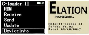
Select **DeviceInfo** to display the Model, Software, and Date information of the device.
