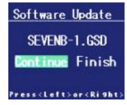
Use  $\longleftrightarrow$  and  $\uparrow \downarrow$  to navigate to the desired file, then press <Enter>  $\biguplus$ . This opens a screen with the file name, and the choice to **Start** or **Return**. Selecting **Start** begins the updating process and a process status screen opens. When this process completes, you are given the choice to **Continue** or **Finish**.
