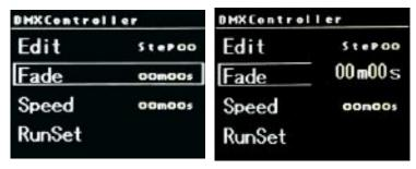
Set **Fade** time by pressing <Enter>  $\rightarrow$  and using  $\leftarrow \rightarrow$  to change minutes, and  $\uparrow \downarrow$  to change seconds.
