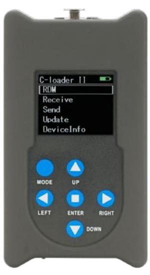
4. Use **MODE** to return to main menu. Use ← → and ↑ to navigate. Select between RDM, Receive, Send, Update, and **DeviceInfo**, then press <Enter> →
