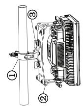
The 32 Hex Panel IP is fully operational in three different mounting positions: hanging upside-down, mounted sideways on trussing, or set on a flat level surface. Be sure this fixture is kept at least 12m (40ft) away from any flammable materials (decoration etc.). ALWAYS use and install and appropriately rated safety cable as a safety measure to prevent accidental damage and/or injury in the event that the clamp fails.
