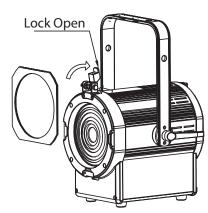
2. Slide the Barn Door in from the top, in front of the Gel Frame. The Barn Door will sit in the same slot as the Gel Frame (Slot 2).
