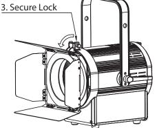
1. Carefully place the FROST FILTER lens on top of the LED lens, making sure it fits securely in place.
