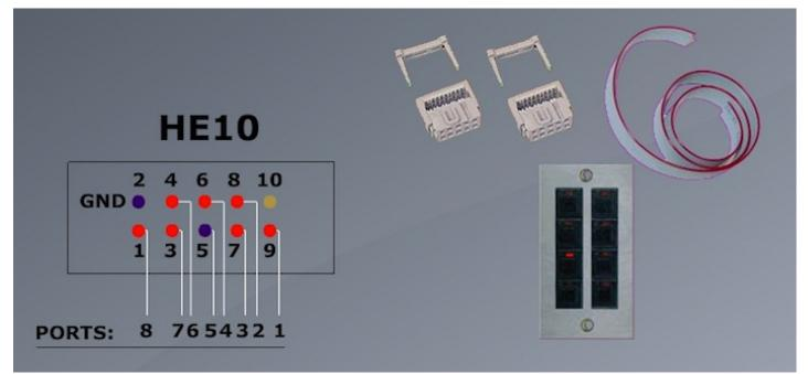
You can connect up to 255 buttons by combining the 8 ports into binary. For example, if ports 1, 2, and 3 are connected to the ground pin, this will trigger address 7.
