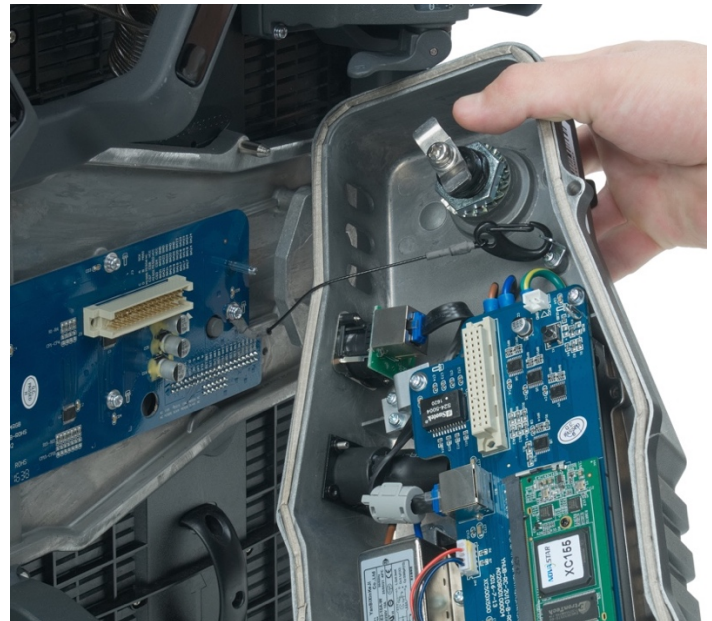
AV3: Power Supply Panel—Opened
