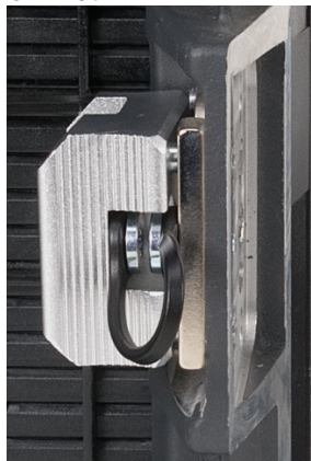
Bottom horizontal tab-keyed connector socket with reversible shim. Place shim inside for straight or convex screen angles (-5° - 0°)
