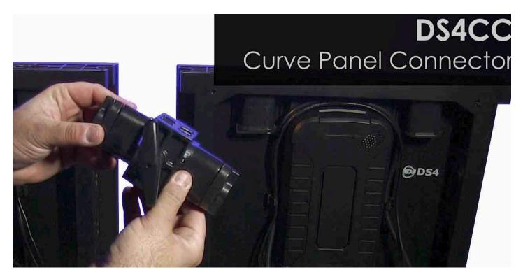
Note the side handle on the DS4CC Curve Connector, which faces the back side of the panels when installed.
