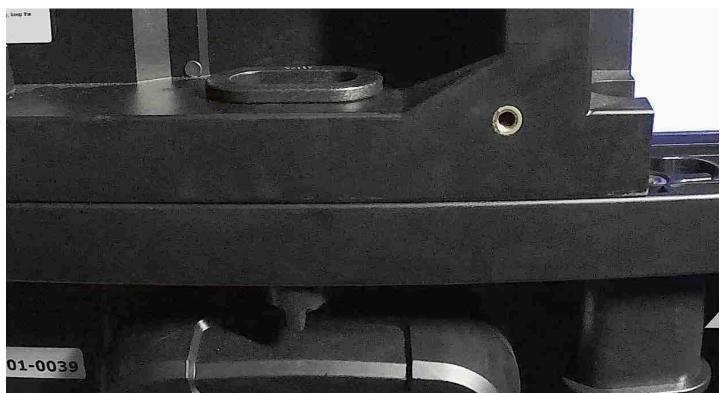
2. With the DS4VC Vertical Connectors installed in both offset panels, twist their locking mechanism knobs to 90° to lock them in place.
