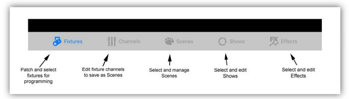
The tabs divide the app into five major sections of workflow. You can move from tab to tab from anywhere within the app by touching a tab icon.
