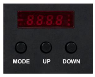
**LED Display On/Off:** To make the display stay ON all of the time press the **MODE** until "**ds-X**" is displayed. Press the **UP** button so that "**ds-1**" is displayed. The LED display will stay ON all of the time. To make the display turn OFF after 10 seconds, press the **UP** button so that "**ds-2**" is displayed. When the LED display turns OFF after 10 seconds, press any button for at least 3 seconds to turn the display on again.
