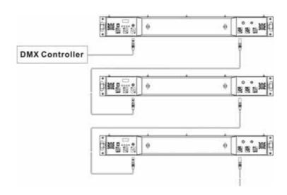
Connect the DMX output of the master fixture in the data chain with the DMX input of first slave fixture. Always connect output with the input of next slave fixture until all slave fixtures are connected.
