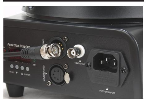
Use a BNC video cable or RCA video cable, with RCA/BNC adaptor, to connect to a video converter or source such as Elations' EPV Image VSC.
